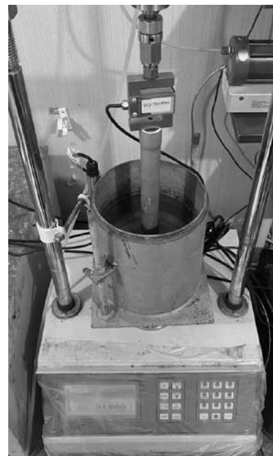
Fig. 2. Open Loop CRS Consolidation Test System Using CBR Mold.
