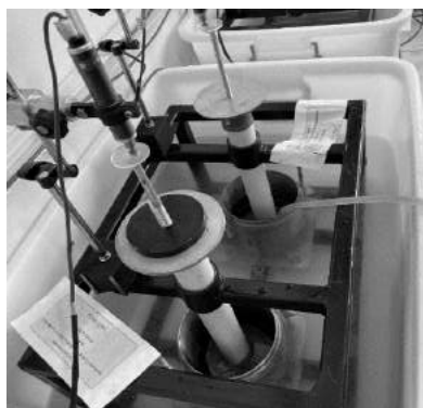
Fig. 1. Incremental Loading Consolidation Test Set Up Using CBR Mold.
