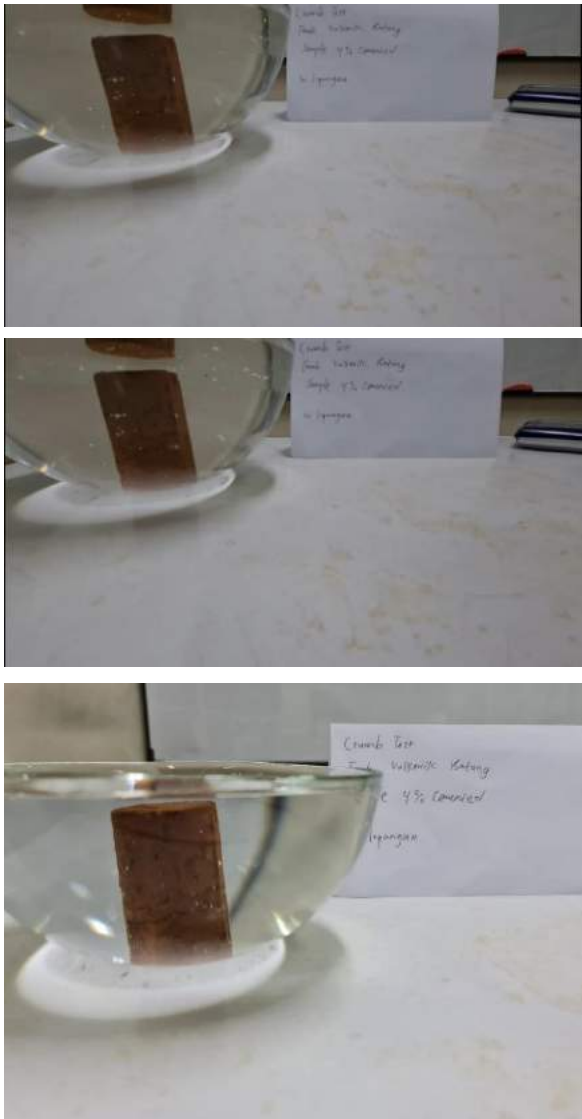
Fig. 8. Batang 4% Cemented Volcanic Soil Crumb Test After 2 Minutes, 1 Hour and 6 Hours.
